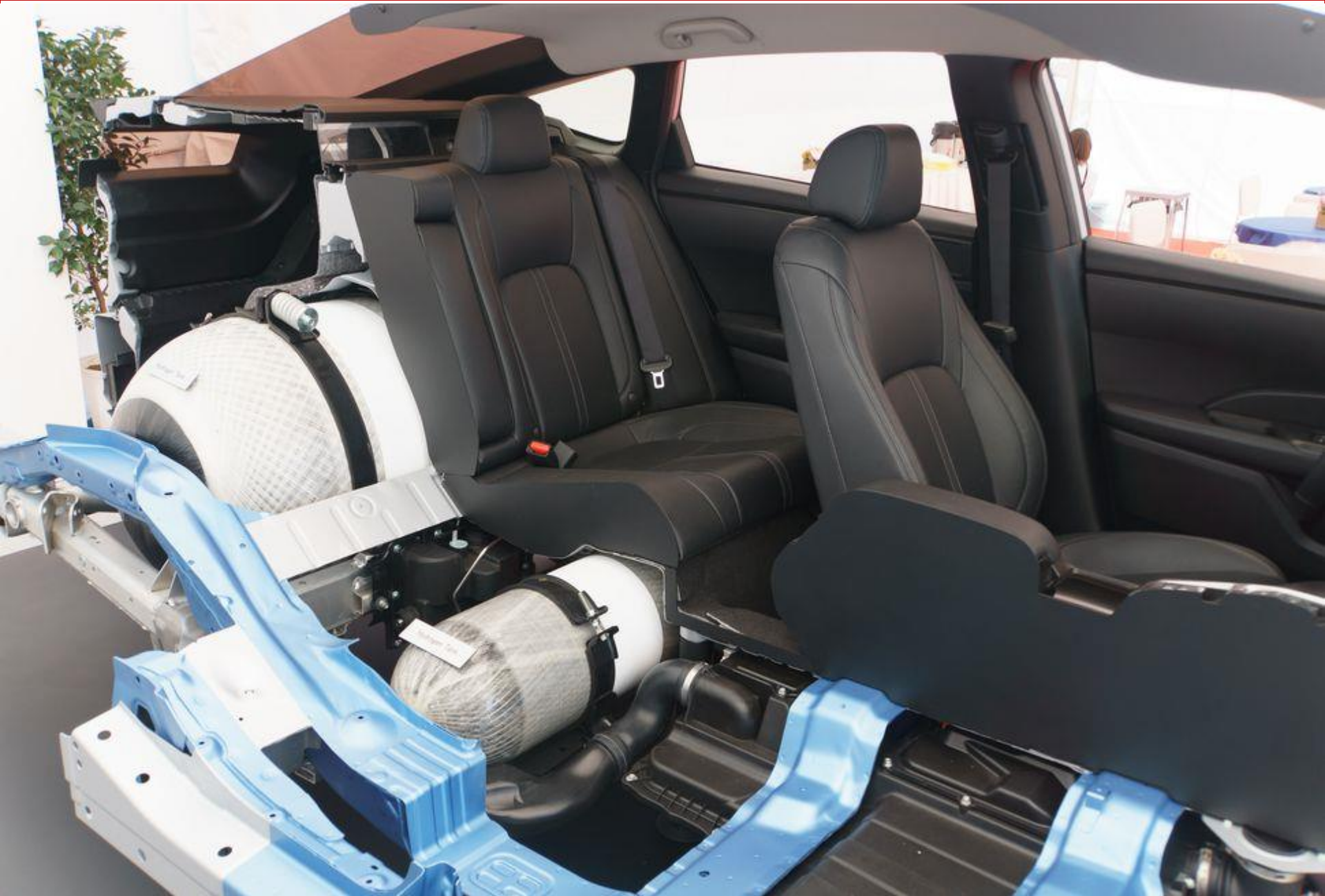
The Clarity's hydrogen tanks fit beneath and behind the rear seats.
